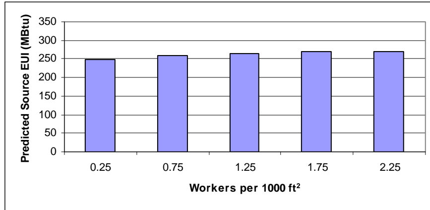
FIGURE 25 – OFFICE – OCCUPANT DENSITY VARIATION 200,000 FT 2 OFFICE, CLIMATE ZONE 12, 80 HOURS/WEEK, 1.25 COMPUTERS/1000FT 2 , 100% HEATED AND COOLED
