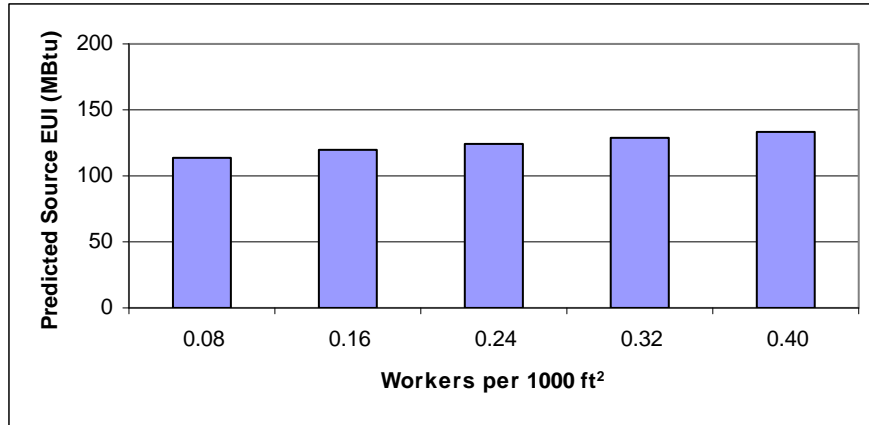
FIGURE 31 – RETAIL – OCCUPANT DENSITY VARIATION 50,000 FT 2 STORE, CLIMATE ZONE 12, 70 HOURS/WEEK, 0.06 COMPUTERS/1000FT 2 , 0.12 REGISTERS/1000 FT 2 , 0.14 REFRIGERATORS/1000FT 2 , 100% HEATED AND COOLED
