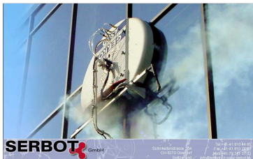
Glass cleaning goes high-tech: The Gekko III Plus is a window-washing robot that can clean approximately 13 times as fast as a manual window washer.
